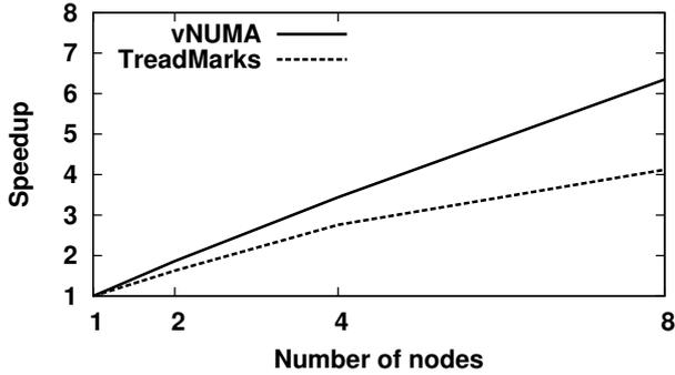
**Figure 3: Scalability comparison of vNUMA and TreadMarks using the Splash-2 [19] “water” benchmark.**
