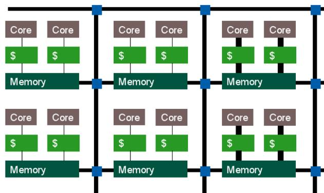
Figure 1: Likely architecture for thousands of cores.
